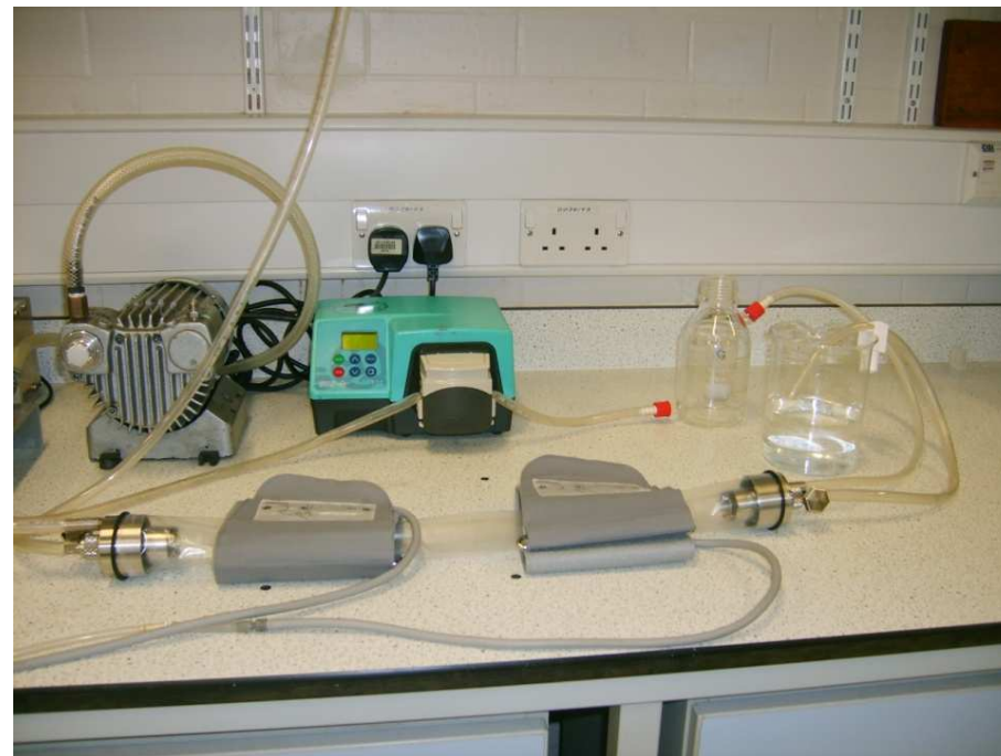
Figure 21: In-vitro small intestine model.
